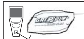
2. Insert key into small hole at top of Gripple. Push in 1/4" to release the cable.
