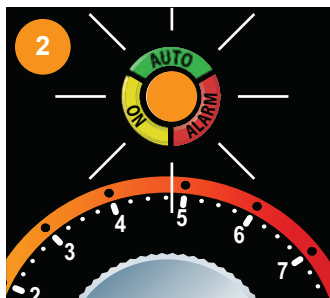
LED light will flash amber rapidly *Early models may have a green continuous blinking light during shutdown sequence.
